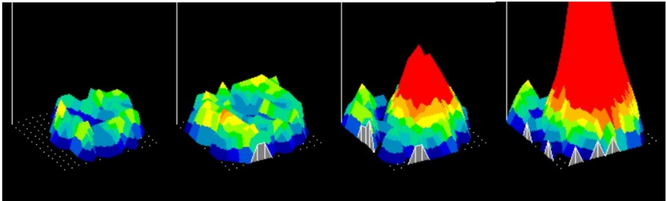
**Figure 5** A short sequence of pressure pad output from a 100 cm drop onto C47, Option 4. The horizontal plane represents the surface of the pressure pad used. The vertical axis represents the pressure recorded.
