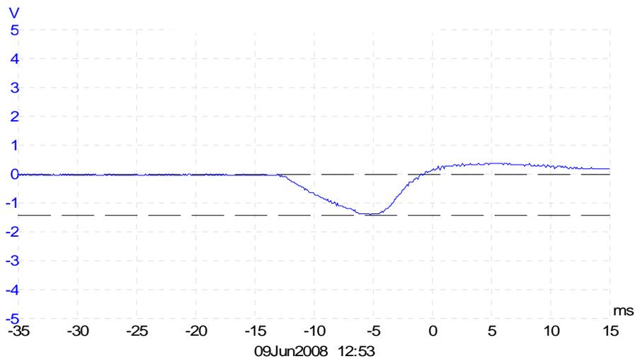
**Figure 3** Typical result where the foam under test was not approaching a “bottoming out” situation. The accelerometer output, V (volts) is plotted against time (milliseconds). Accelerometer sensitivity is 27.44 millivolts/g.
